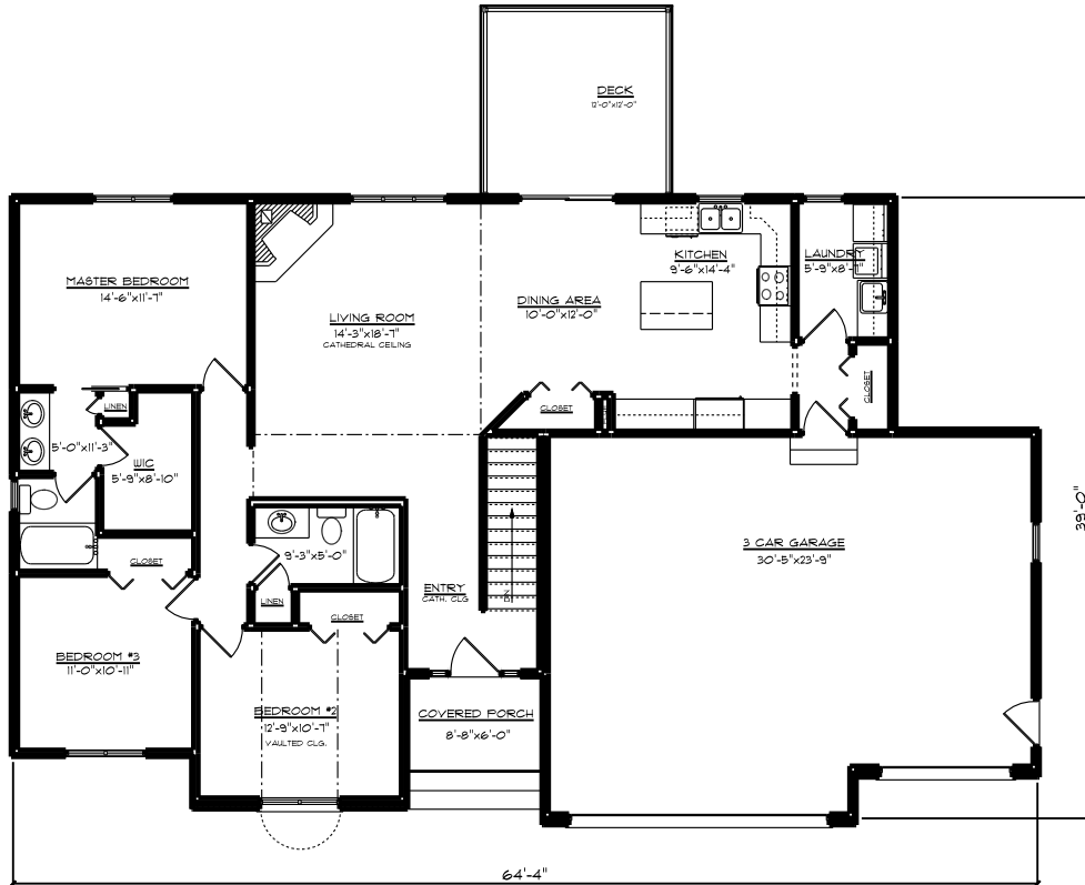
MAIN LEVEL FLOOR PLAN MAIN LEVEL SQ. FT.: 1497 SQ. FT. TOTAL FINISHED SQ. FT.: 1497 SQ. FT.
